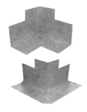
Flexible system component made from Ceratec DF1 DEB sealing and decoupling membrane with double-sided fleece coating, used within bonded waterproofing systems in accordance with DIN 18534. Crack-sealing, alkali-resistant, ageing-resistant, made from tear-resistant polyethylene.
