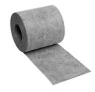
Flexible system component made from Ceratec DF1 DEB sealing and decoupling membrane with double-sided fleece coating, used within bonded waterproofing systems in accordance with DIN 18534. Crack-sealing, alkali-resistant, ageing-resistant, made from tear-resistant polyethylene.
